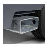
Easy to move Loading and unloading the Drillair compressor is easy thanks to the forklift slots.
