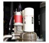
Extend the lifetime of your equipment The new OilXpert prevents condensation in the oil system, extending the lifetime of the bearings and element. The OilXpert application is CANbus controlled.
